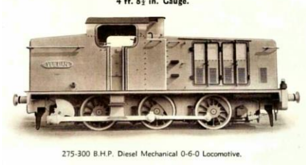
275-300 B.H.P. Diesel Mechanical 0-6-0 Locomotive.
